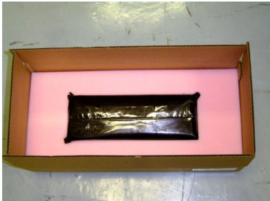
Power supply was placed in bag. The bag was then "wrapped" around the power supply, sealed with tape, and inserted into carton as shown.
