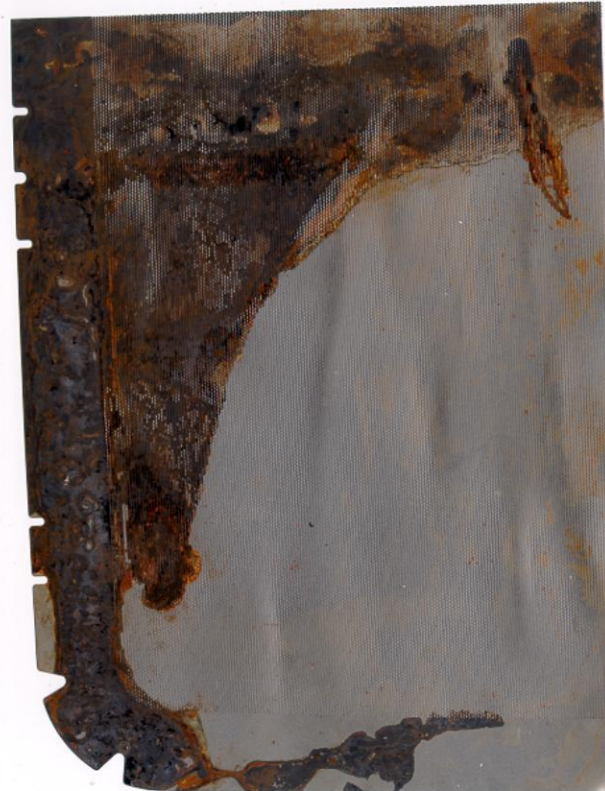
Tightly Over-Wrapped W/0.006" VCI Kraft paper and Heat Sealed in a 0.003" LDPE Bag
